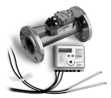
The Supestatic 440 is the heat and cooling meter with the most complete range of flows in the heat meter industry, from DN15 - DN 500 and qp 1 – qp 1500 respectively. The unique static measuring principle of fluidic oscillation without moving parts in the pipe and the robust design ensures a precise, stable and reliable measuring of flow over a long time.
