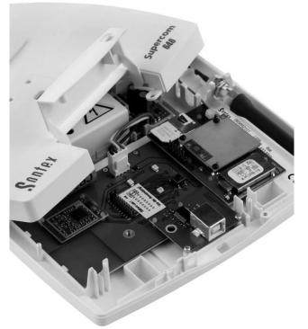
As the radio central Supercom 646 is also available with an M-Bus module, e.g. an existing M-Bus network can be easily extended with a radio network and the radio measuring devices will be directly read from an M-Bus central. The radio central becomes an M-Bus participant (slave) in an M-Bus network.
